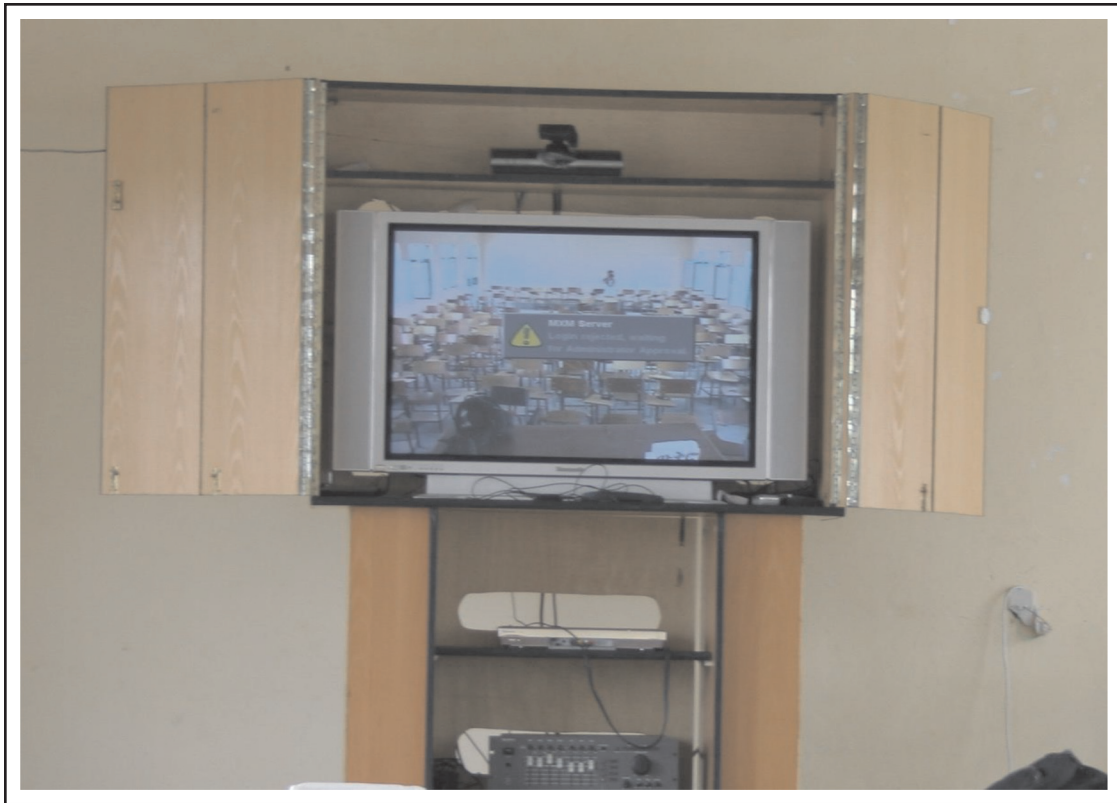
Figure 1. The Woredanet equipment, composed of, from top to bottom, a videocamera, a plasma TV screen, a decoder, and an amplifier/equalizer.
